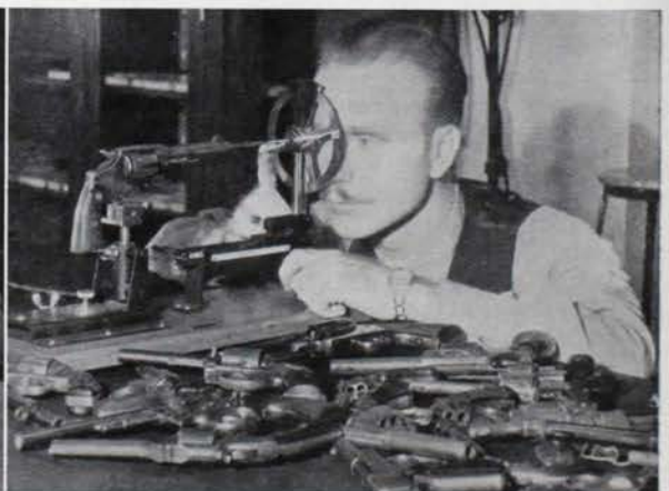
The use of the helixometer for fire arms identification, commonly referred to as ballistics.
