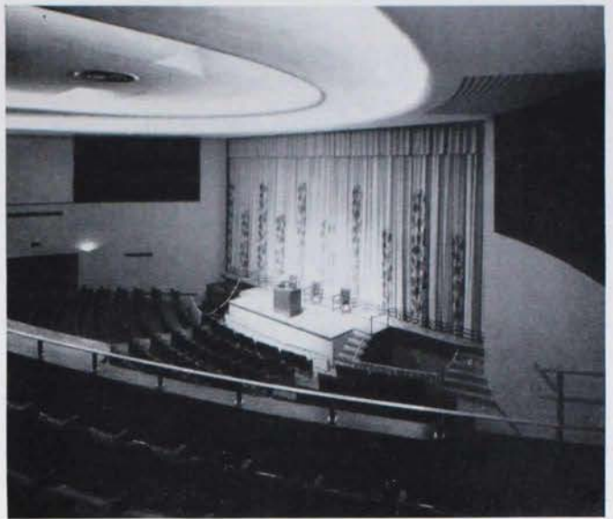
Wide and comparatively shallow, the Cahn Auditorium permits maximum facilities for seeing and hearing from all seats on the main floor and in the balcony. The entire speakers' unit is removable.
