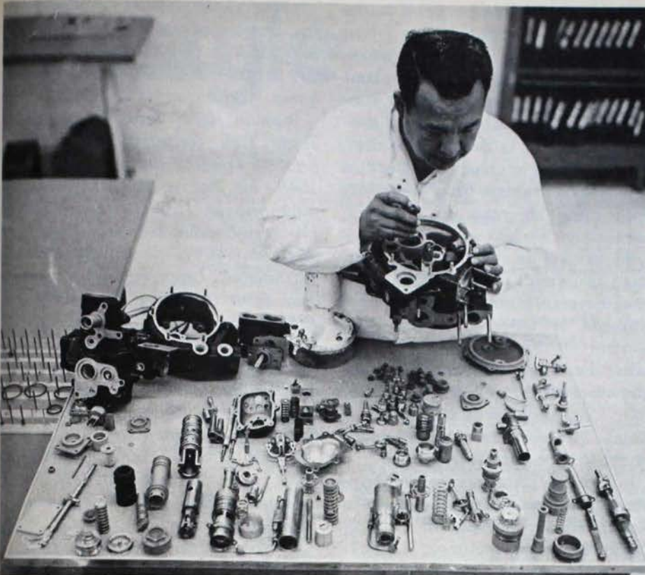
Overhauled fuel controls are reassembled under controlled atmospheric conditions.
